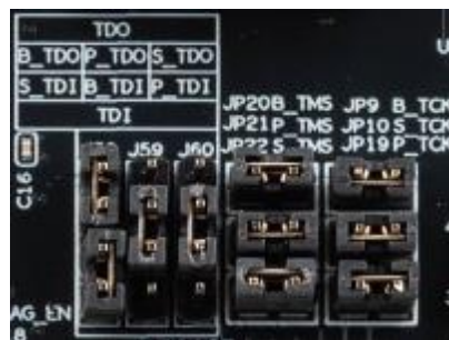
Figure 4.1. Default JTAG Chain Jumper Setting
